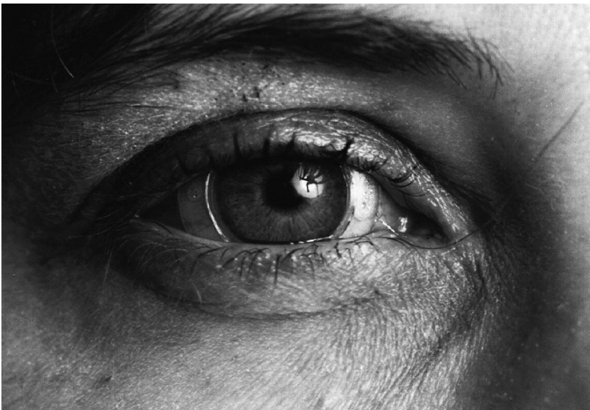
Figure 1-1. The scleral search coil method for precise measurement of horizontal, vertical, and torsional eye rotations. The subject is wearing a silastic annulus in which are embedded two coils of wire, one wound in the frontal plane (to sense horizontal and vertical movements) and the other wound in effectively the sagittal plane (to sense torsional eye movements). When the subject sits in a magnetic field, voltages are induced in these search coils that can be used to measure eye position (see Appendix B for details).
